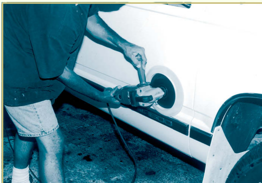
FIGURE 10—High-speed, 90-degree Electric Buffer
