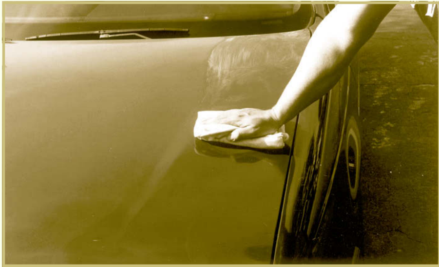
FIGURE 11—Buffing a Finish by Hand
