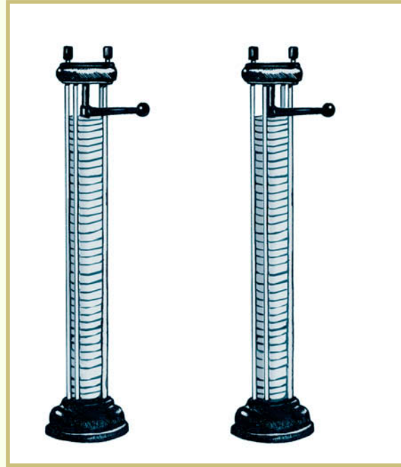
FIGURE 6 —The voltaic pile was originally invented to generate electricity.
