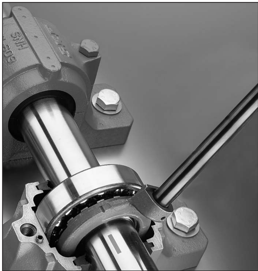
FIGURE 28 —Spanner wrenches are often used to install and remove shaft nuts. (Photo Courtesy of SKF USA Inc.)
