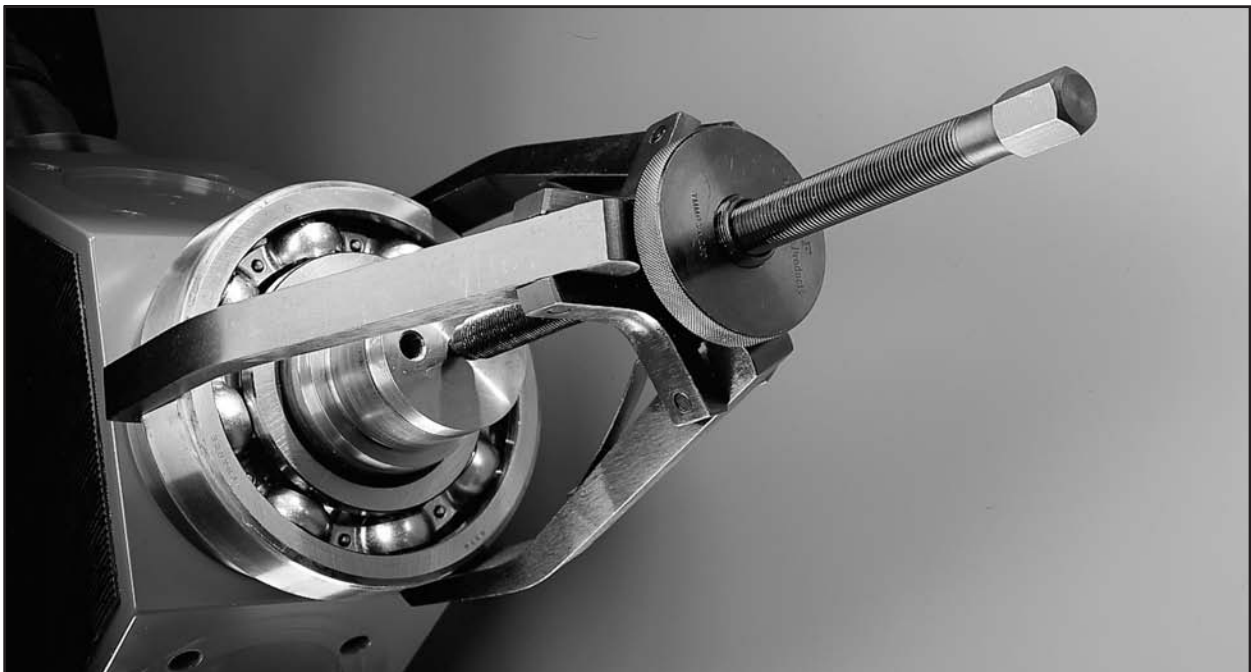
FIGURE 27 —Careful removal of antifriction bearings is important. Here a bearing puller is used. (Photo courtesy of SKF USA Inc.)
