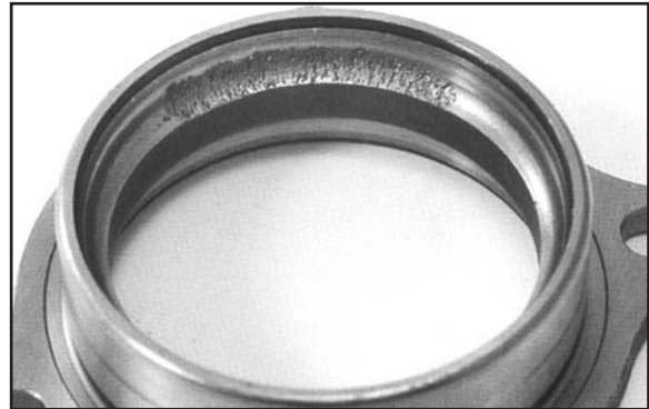
FIGURE 24 —This damage was caused by poor installation. (Courtesy of NTN Bearing Corporation of America)
