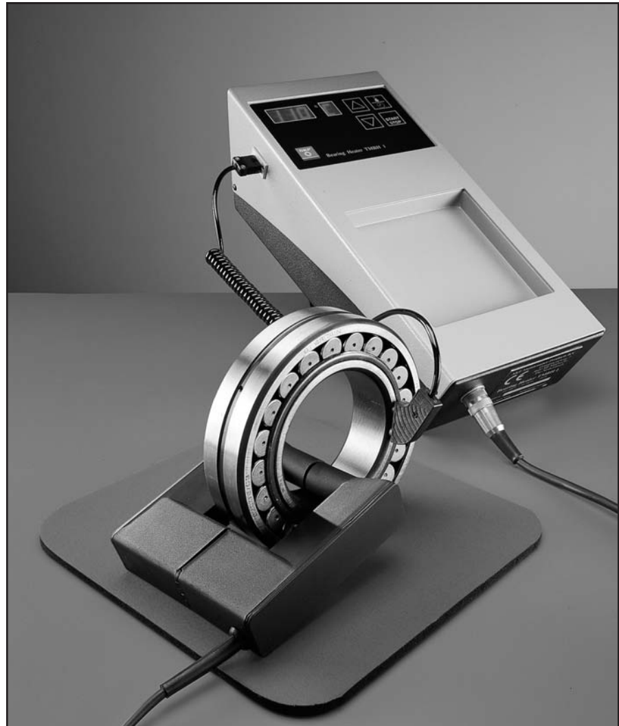
FIGURE 20—Bearings can be heated with an induction heater to ensure uniform and highly controlled thermal growth. (Photo Courtesy of SKF USA Inc.)
