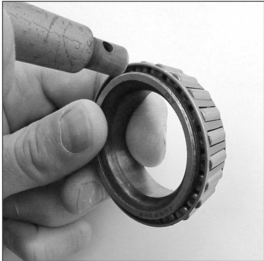
FIGURE 29 —When using pressurized air to clean a bearing, be sure that the bearing isn't allowed to spin.
