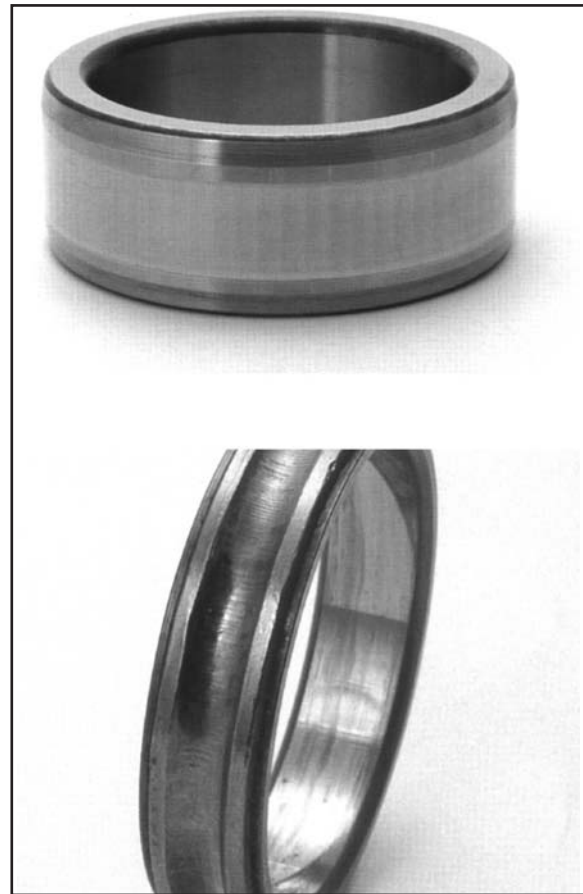
FIGURE 31—These races were damaged by vibration. (Courtesy of NTN Bearing Corporation of America)
