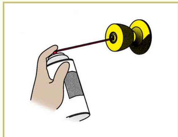
FIGURE 7—Lubricating a Lock
